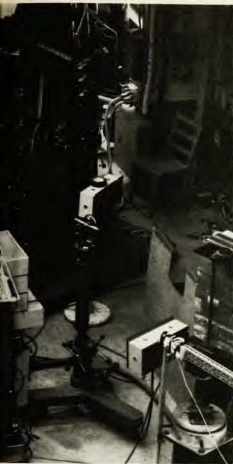
Apparatus for neutral K-meson experiment. Housings contain spark chambers and cameras. Researcher is standing near the triggering system electronics. (Photograph courtesy of Brookhaven National Laboratory).
