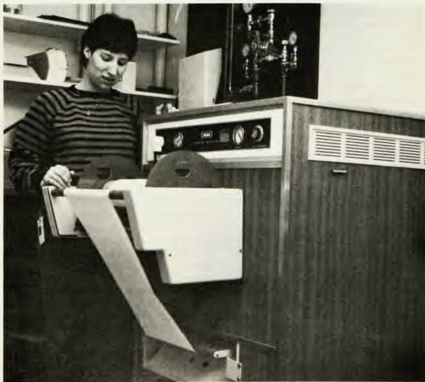
Galley production: developer for processing the photographic output of the Videocomp electronic composer; it produces galleys for both ATEX and UNIX computer composition systems.
