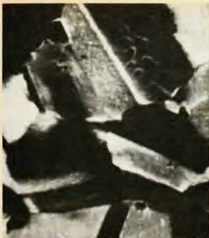
Striking crystallographic contrast , strongly dependent on the angle of beam incidence, is seen in these two scanning ion micrographs of the same sample of recrystallized brass. At left, the scanning beam of gallium ions strikes the polished sample surface at normal incidence; at right, the beam is tilted 10°. Light and dark regions are reversed. The high contrast and its directional dependence are attributed to channeling of the ions between crystal planes, affecting the strength of the secondary electron signal that generates the image. Micrographs by University of Chicago group. Full scale is 64 microns; resolution is 1000 Å.
