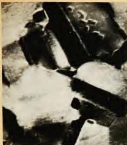
Striking crystallographic contrast , strongly dependent on the angle of beam incidence, is seen in these two scanning ion micrographs of the same sample of recrystallized brass. At left, the scanning beam of gallium ions strikes the polished sample surface at normal incidence; at right, the beam is tilted 10°. Light and dark regions are reversed. The high contrast and its directional dependence are attributed to channeling of the ions between crystal planes, affecting the strength of the secondary electron signal that generates the image. Micrographs by University of Chicago group. Full scale is 64 microns; resolution is 1000 Å.
