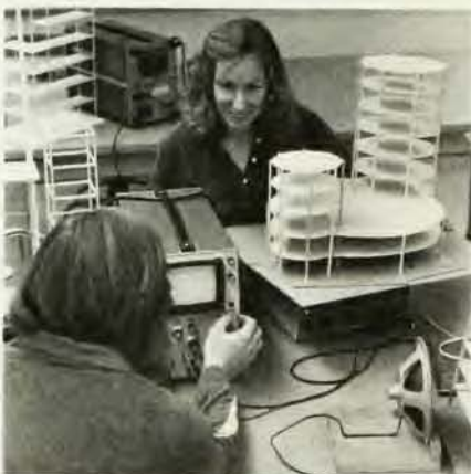
Architectural models are shaken by Cal Poly students Elizabeth Fisher and Douglas Maze with the "earthquake spectrometer," which uses Lissajous figures to monitor the amplitude and phase of the resonances of the structure. (Photo by Brad Hartwell.)
