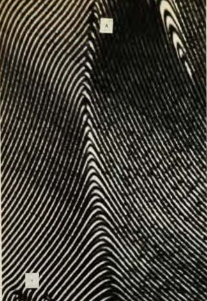
Inside a focal conic defect in a cholesteric liquid-crystal polymer. 11 This slice through the defect is shown as it appears when held between crossed polarizing filters. The distance between two "stripes"—about 2 microns here—is a half pitch, as illustrated in the figure on page 40. This is the cholesteric analog of the smectic layer. As the cholesteric planes turn to line up with the polarizers, the contrast changes. A strong maximum in the twist axis occurs at A. The further the slice is from the focal line, the weaker this curvature. At I there is a dislocation composed of two \lambda defects, of strength \frac{1}{2} and -\frac{1}{2} . Figure 6
