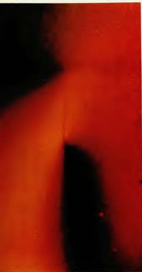
Thin-thread defect "frozen" by polymerization in the nematic phase and placed between crossed polarizers for observation. As the schematic diagram below shows, in the region of the thread each slice of the sample contains a point at which the direction of the long axes of the molecules varies discontinuously. The thin-thread defect is the locus of such singular points. Figure 2
