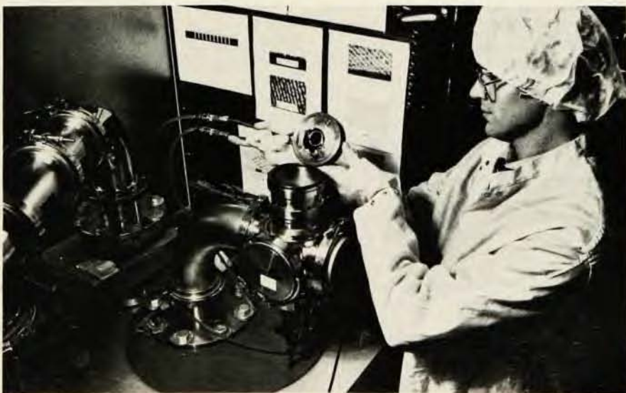
At the Submicron Structures Lab at MIT, the x-ray lithography station, shown above being loaded by Andrew Hawryluk (visiting from the University of Florida), is used to make structures on the order of hundreds of angstroms. An x-ray beam strikes a chip masked with a thin membrane of metal.
