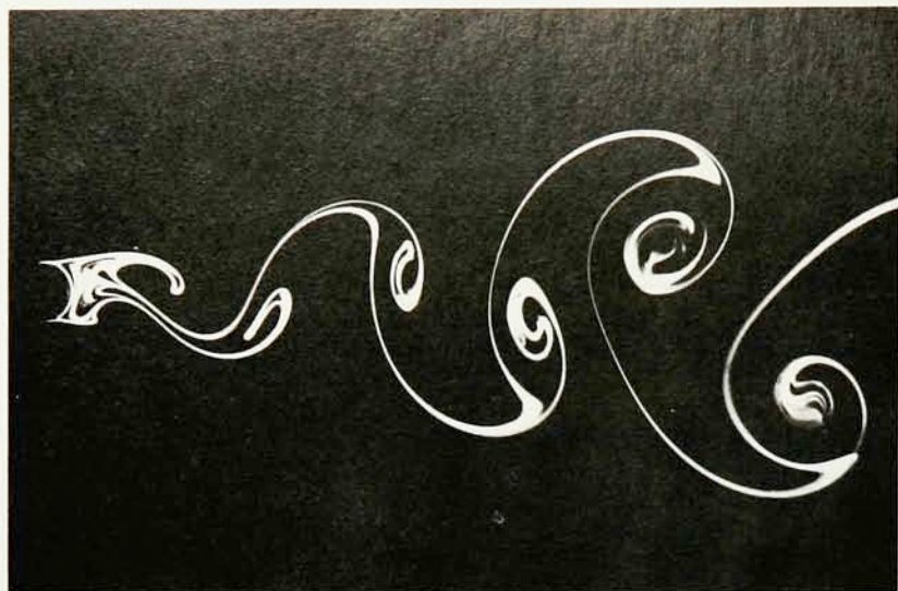
Kármán vortex street behind a circular cylinder. This is one of over 200 photographs collected in An Album of Fluid Motion by Milton Van Dyke (176 pp. Parabolic Press, Stanford, Cal., 1982. $20.00 cloth, $10.00 paper). Designed as a supplement for students and teachers of fluid mechanics, the book contains pictures from around the world, organized generally to go from low speeds to high, from creeping flows to shock waves and hypersonic flight. The photograph above, taken by Sadatoshi Taneda, shows water flowing at 1.4 cm/sec past a cylinder 1 cm in diameter, with R = 140 . Integrated streaklines are shown by electrolytic precipitation of a white colloidal smoke illuminated by a sheet of light. The vortex sheet is seen to grow in width downstream for some diameters.
