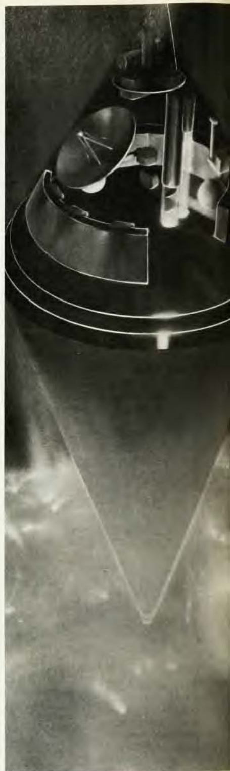
Starprobe encounters the Sun. Artist's conception shows the spacecraft's primary thermal shield, which has a central aperture that allows instruments to image the Sun. Other instruments image the back-scattered light of the corona outside the trajectory of the spacecraft. A package of magnetic-field and particle-detection instruments (top) is mounted on a spinning platform at the apex of the volume that remains shaded by the primary shield at perihelion. The final major group of instruments is a drag-free subsystem that allows a precise determination of the spacecraft's orbit. (Courtesy of James Randolph, Jet Propulsion Laboratory.)
