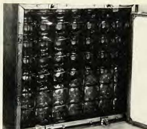
Position-sensitive neutron detector developed at Argonne for the single-crystal diffractometer at the IPNS I spallation source. A 7 \times 7 array of photomultipliers is behind a panel of Li 6 -loaded glass (not shown). The position of a neutron interacting in the glass is determined with a spatial resolution of 3 mm.
