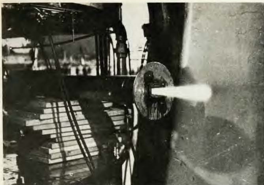
Cyclotron beam. The ion beam from the 60-inch cyclotron exits the vacuum chamber through a window, ionizing the air in its path and producing a beautiful purple glow.
