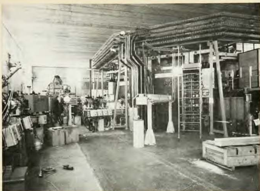
The GANIL heavy-ion facility is a tandem system of two large room-temperature cyclotrons capable of accelerating light ions to 100 MeV/nucleon, and uranium to 10 MeV/nucleon. Each has an extraction radius of 3 meters. Shown here is the first cyclotron.
