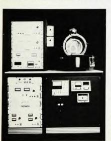
oxide and silicon masks. The TLA 20-M permits totally dry processing of conventional positive and negative photoresists, as well as electron beam resists such as PMMA, COP, PBS and iodinated polystyrene. Technics IMF, 7950 Cluny Court, Springfield, Virginia 22153
