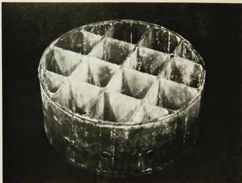
Honeycombed pyrex mirrors produced at the University of Arizona are being considered for the next generation Multiple Mirror Telescope. Test casting seen here without faceplate.
