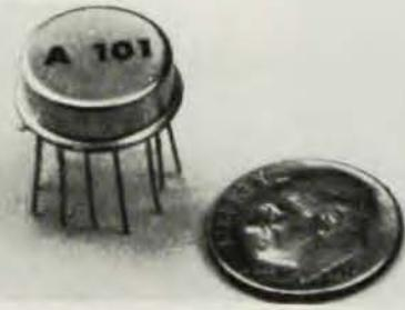
Model A-101 is a Charge Sensitive Preamplifier-Discriminator and Pulse Shaper developed especially for instrumentation employing photomultipliers, channel electron multipliers and other charge producing detectors in the pulse counting mode. Its small size (TO-8 package) allows mounting close to the collector of the multiplier. Power is typically 15 milliwatts and output interfaces directly with C-MOS and TTL logic. Input threshold and output pulse width are externally adjustable.
