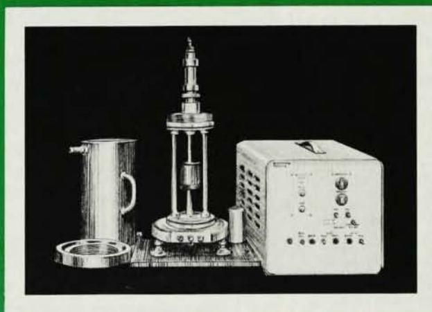
Coal Research—measures volumetric changes as a function of temperature at elevated pressure.
