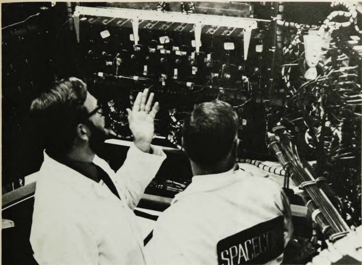
Interior of TDRSS satellite shows signal multiplexer, right; transmitter for the multiple access phased array antenna (vertical white stakes in cover photograph), center; and C-band system for domestic telecommunications, left. James Wertz (left), who worked in technical management on the Tracking and Data Relay Satellite System project, is
