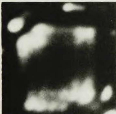
Images of large clusters of adatoms on the (110) plane of tungsten show the beginning of a new atomic layer. Shown in these photographs taken by H.-W. Fink, are large clusters of palladium and iridium adatoms (top), and platinum and silicon adatoms (bottom). These adlayers are not densely packed and the symmetry of the atomic arrangement is not the same for all. Individual atoms in the adlayers are so widely spaced that they can be resolved; the (110) substrate surface, in contrast, is densely packed and appears dark and featureless. Figure 7
