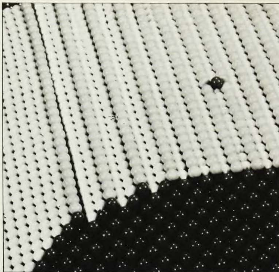
Hard-sphere model of a body-centered cubic lattice reveals a variety of atomic arrangements on different crystal planes. A single adsorbed atom residing on the surface is represented by the sphere on the (211) plane. Figure 2
