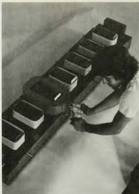
Wiggler magnet for SPEAR (lower half) with seven full poles and two end half poles. Each pole is powered by a coil, only one of which is shown. (Photo by J. Faust, SLAC) Figure 5.
