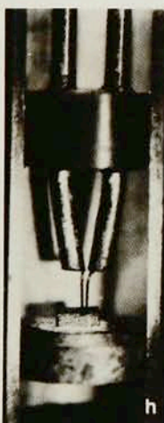
(g) Walter Brattain's laboratory notebook and (h) one of the first transistors.
