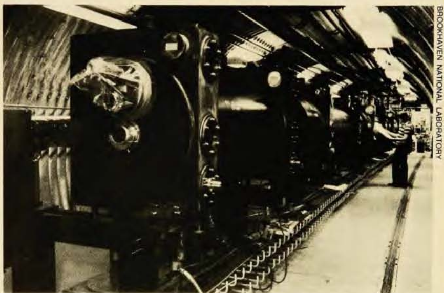
Mock-up of a section of the Isabelle tunnel , showing a string of superconducting magnets. Problems with the development of superconducting magnets for both Isabelle and the Energy Saver need to be solved, according to a report to the High Energy Physics Advisory Panel.
