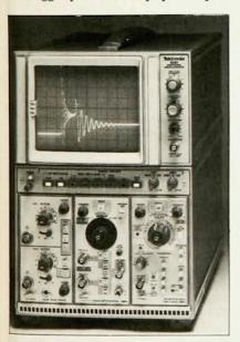
100 microsec/division. The bislope triggering, which lets the user select a trigger voltage window, serves to eliminate missed trigger events; single-shot data are easily captured. Bislope trig-
