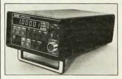
other nanovoltmeter currently available. It provides 5½ to 6½ digit resolution, with a one-standard-deviation sensitivity of 10 nV.
