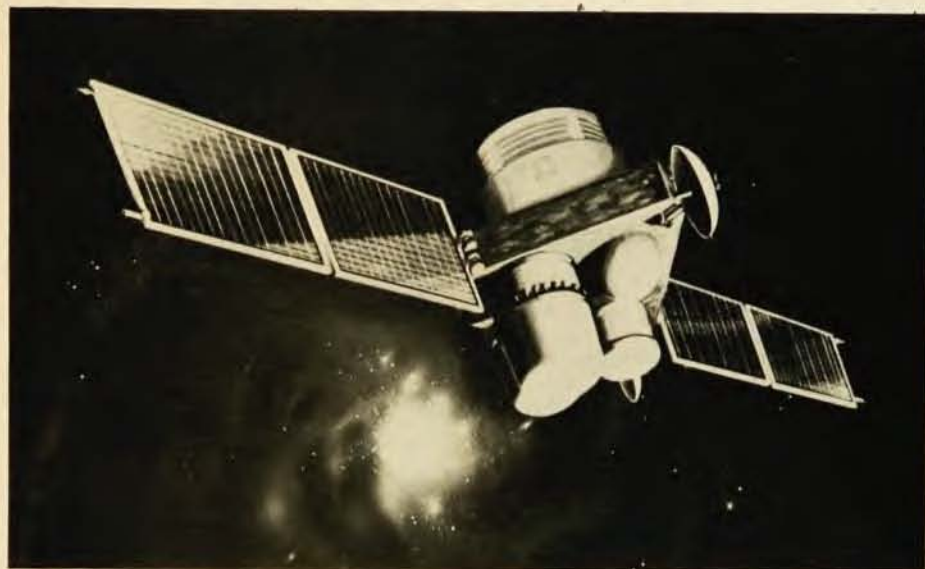
Gamma Ray Observatory , to be launched in 1985, will carry a high-resolution spectrometer, burst detector, broad-band spectrometer, double Compton telescope and high-energy telescope.
