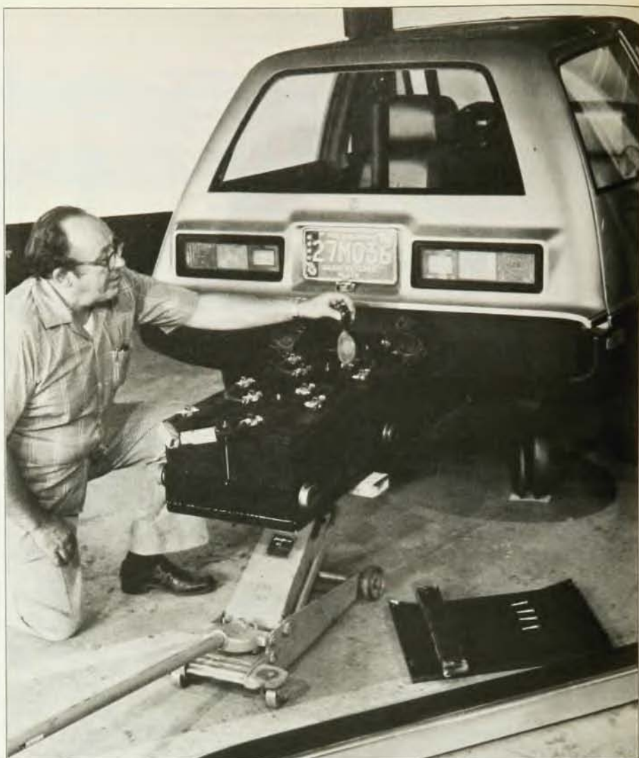
A four-passenger electric car being loaded with advanced lead-acid batteries. It is designed for urban driving, and has a range of about 45 miles. (Photo courtesy of General Electric.)
