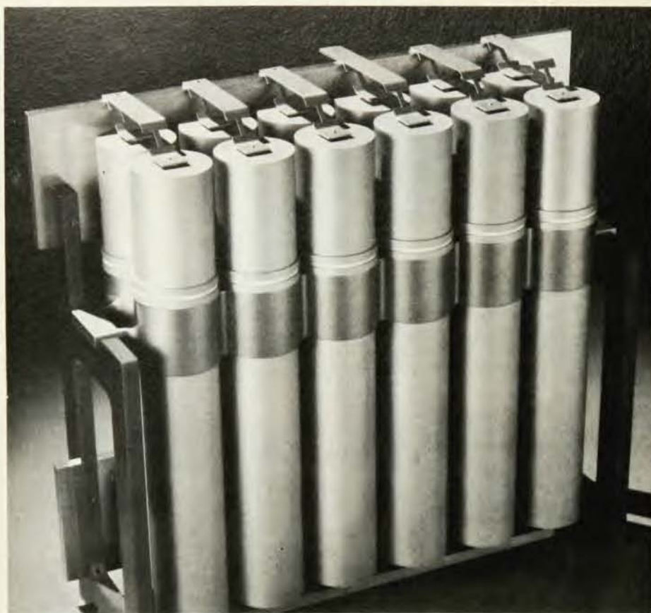
Sodium-sulfur battery pack (experimental model). The batteries operate at 300–375° C. (Photo courtesy of Ford Motor Co.)
