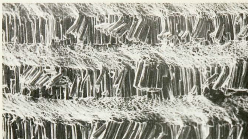
Multilayer sputter deposit of a metal (Ni—50 Cr) and a ceramic (ZrO 2 ). This photograph of a fracture surface shows a section about 0.2 mm wide. Figure 7
