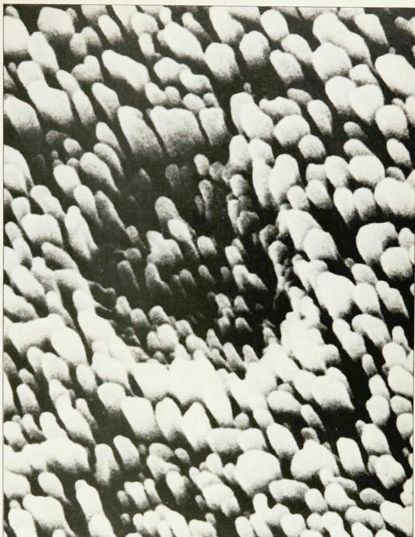
Columnar structures on a beryllium surface. These 500-nanometer-high features are examples of the complex surface morphology that can occur when materials are bombarded by ions at a flux of about 2 \times 10^{21} ions \text{cm}^{-2} . (Sandia National Laboratories scanning-electron micrograph from a study conducted by J. K. G. Panitz, D. J. Sharp and J. T. Healey.) Figure 1
