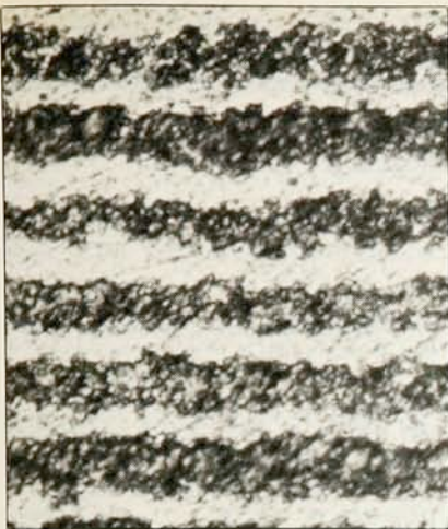
Polished and etched surface of a multilayer vacuum deposit of alternating layers of copper (50%) and nickel (50%) fabricated by dual-source evaporation. Figure 8
