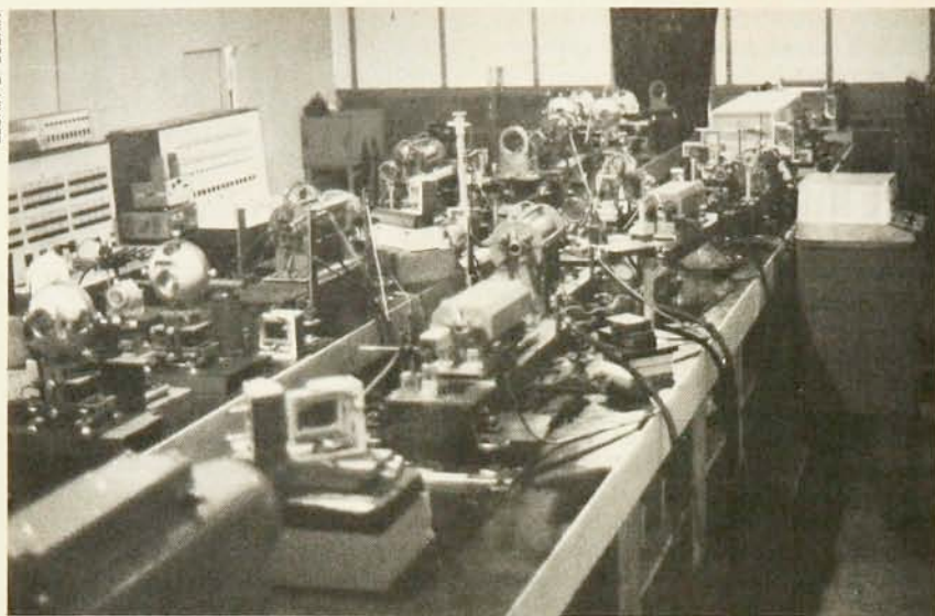
Six-beam neodymium-glass laser is being used for inertial-confinement experiments at the Shanghai Institute of Optics and Fine Mechanics. Each beam produces 100 GW in 1 nanosec.
