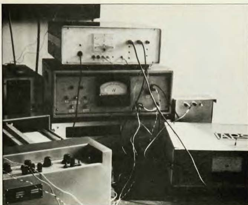
X-ray appearance potential spectroscopy (APS) equipment at Fudan University. Hua Chung-yi recently spoke at the American Vacuum Society meeting on experiments with the equipment.
