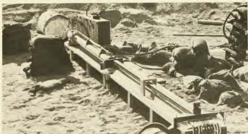
Livermore-Los Alamos rail gun at the Los Alamos firing site. Two 8-foot-long parallel copper strips (foreground) constitute the magnetic-flux-compression generator. Sheet explosive driving the upper strip down generates a megawatt current pulse in the 6-foot-long small-bore rail gun (background). The \frac{1}{8} -inch plastic cube is launched at speeds up to 5.5 km/sec.
