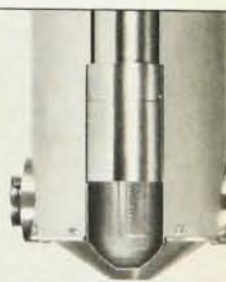
Direct measurement of molecular beam flux from each furnace at deposition position
