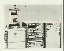
density and fine resolution. It can polish substrates and deposit high-quality thin films by ion-beam sputtering. One can use both inert and reactive gases, so that both direct-beam physical and chemical etching can be undertaken.
