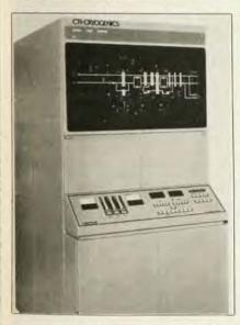
at rates up to 60 liters per hour. The model 2800 can be used as a helium liquifier or as a closed-cycle 4.5-K refrigerator. It can also perform the two roles in combination. It is designed for long-term, unattended operation.
