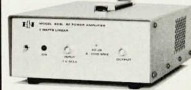
With a flat frequency response and 3 watts of linear Class A output (up to 5 watts saturated), the 603L will provide constant forward power, making it ideal for driving reactive or resistive loads.
