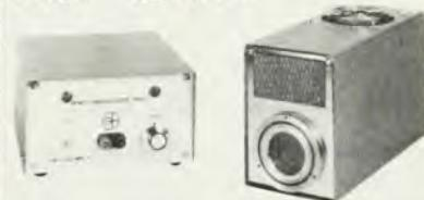
Compact, lightweight, with low power requirements. Forced air-cooled to -30° with 20° ambient. Temperature can be pre-set and controlled to 0.5°C. Dew Free.
