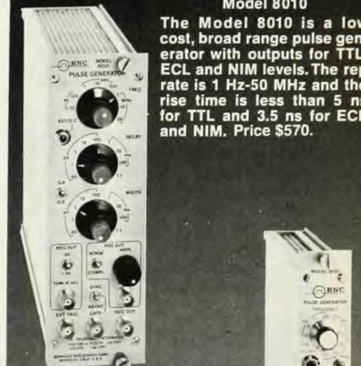
The Model 8010 is a low cost, broad range pulse generator with outputs for TTL, ECL and NIM levels. The repetition rate is 1 Hz-50 MHz and the rise time is less than 5 ns for TTL and 3.5 ns for ECL and NIM. Price \$570.
