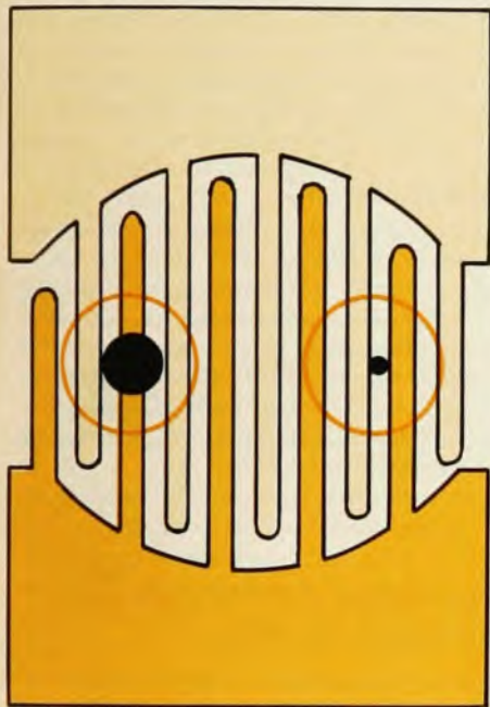
Schematic of interdigitated electrodes produced on diamond flat. Actual electrodes have 75 or more fingers. A thin sample is put on top of electrodes. Dashed circles show the circumference of the contact circle when the indenter is applied. Black center circles show two possible cases in which the sample has become conducting.
