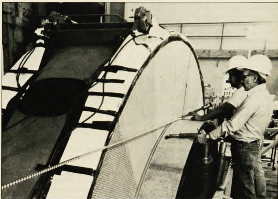
Construction of superconducting coils for MFTF at Livermore. Initial lengths of superconductor are being wound on coil form, which has been prepared with Kapton and perforated G-11 sheet. Also visible is the interturn spacer strip attached to the superconductor to insulate its layers.
