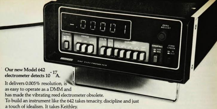
Voltage reading capability is  $10 \,\mu\text{V}$  to  $10 \,\text{V}$  with  $10^{16} \,\Omega$  input resistance. Charge is measurable from  $4 \times 10^{-16} \,\text{C}$  to  $10^{-10} \,\text{C}$ ; input current is only  $5 \times 10^{-17} \,\text{A}$ . Zero to 99% response time is 100 ms on  $10^{-10} \,\text{A}$  ranges, and 400 ms on  $10^{-11} \,\text{A}$  ranges.
