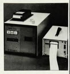
and the open end sealed with a 6-µm polyester film. The sample is placed, film side down, over the window of the probe head located on top of the instrument. With the shield of the probe head closed, the sample is exposed to x rays from an encapsulated Cd-109 radioisotope source contained in the instrument head. The resulting fluorescence x rays are analyzed by energy dispersive detection and analysis.—
