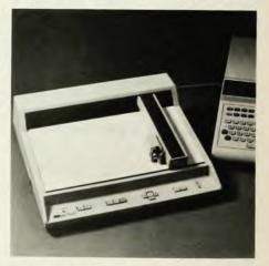
lines. Fast continuous plotting is provided by drawing between points at 250 mm/s. Text can be drawn at speeds up to three characters per second for annotation. A modular interface system allows change between various interfaces. The mechanical system is based on a linear stepper mechanism.—Hewlett-Packard Company, 1507 Page Mill Rd., Palo Alto, CA 94304.
