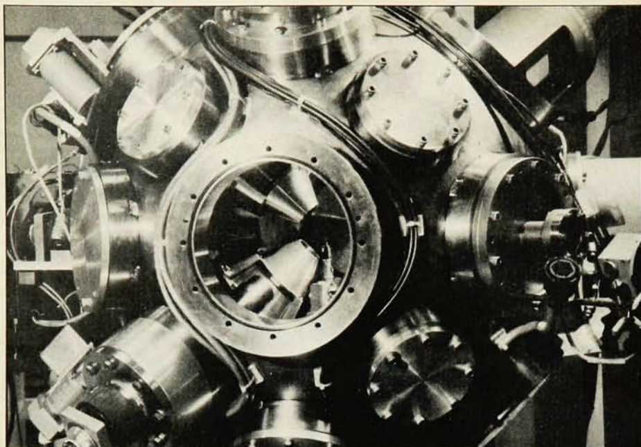
Interim target chamber at the University of Rochester Laboratory for Laser Energetics uses the six beams of the Zeta neodymium-glass system. In December, 24 beams are expected to operate.
