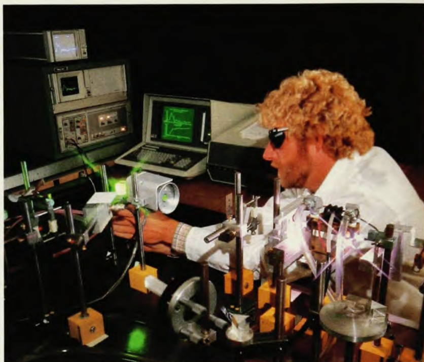
A Tektronix Signal Processing System monitoring a repetitively pulsed ND:YAG Laser and frequency doubler at the Oregon Graduate Center for Study and Research
