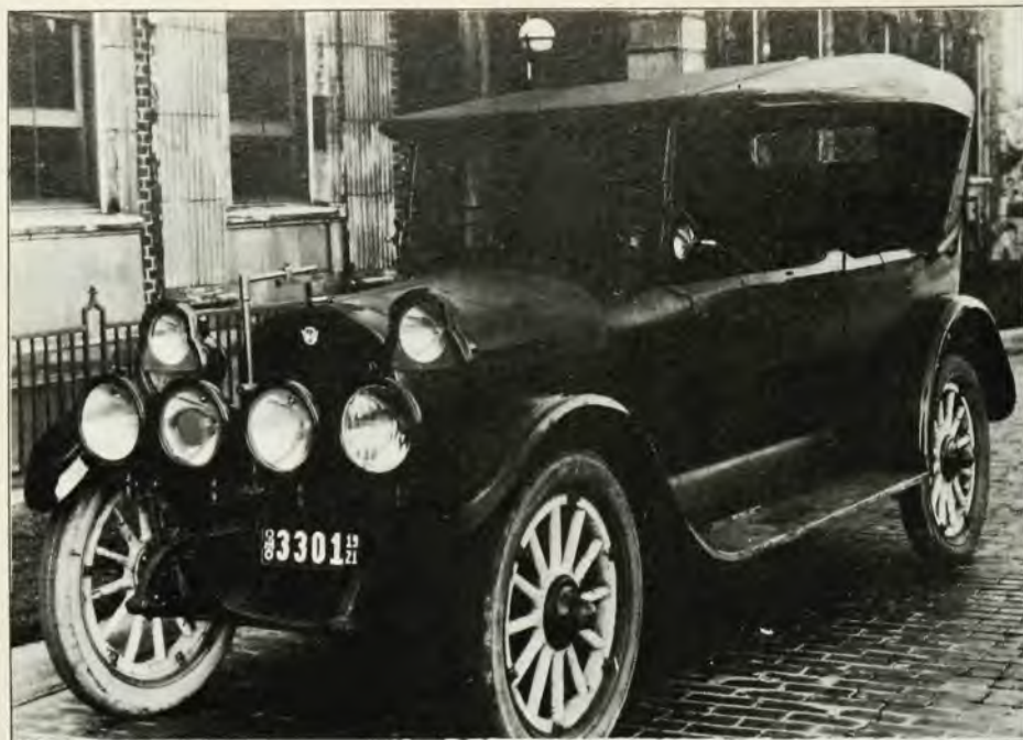
Test vehicle for lamps. This 1920 Reo touring car was one of General Electric's "laboratories on wheels" for testing headlamps as well as other lights for automobiles. (General Electric Co.)
