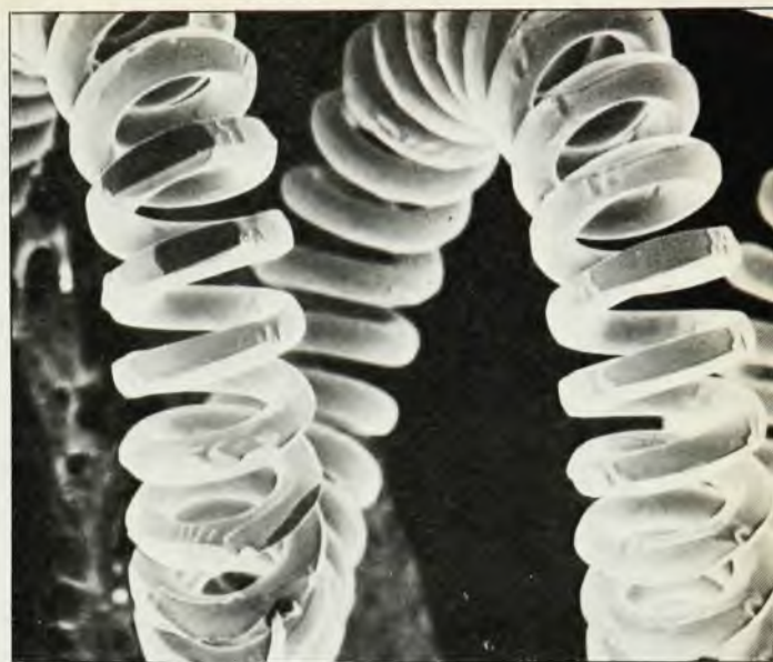
Coiled-coil tungsten filament. On the left is a scanning-electron micrograph of a filament from a conventional 100-W lamp, fresh from the factory. On the right is similar filament from a bulb that had burned for about 500 hours. Note the growth of crystal structures, outlined by thermal etching, and the start of a few offset fractures; some of the crystals extend over several coils. (SEM photos by H. F. Webster.)
