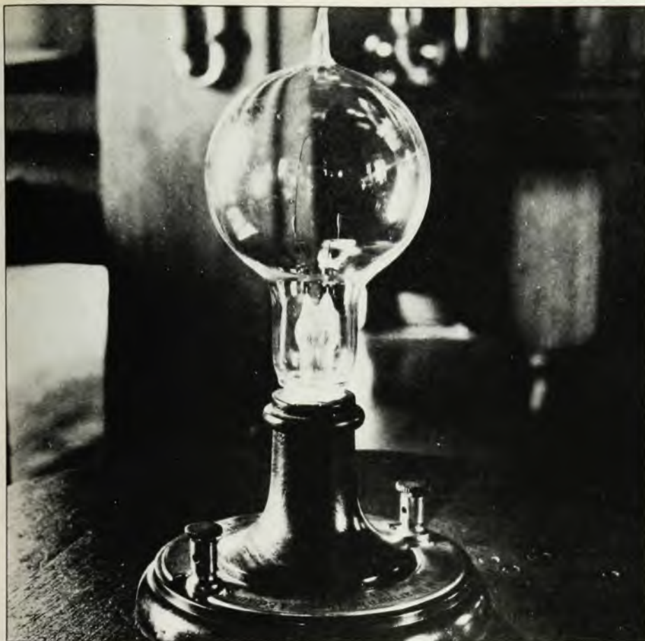
Replica of the first electric lamp. Its filament is a carbonized sewing thread. Edison himself made the replica in 1929, at a celebration of the fiftieth anniversary of his original achievement organized by Henry Ford in Dearborn, Michigan. Edison's lab was moved to a nearby site and restored for the occasion. (Photo courtesy of US National Park Service, Edison National Historic Site.)
