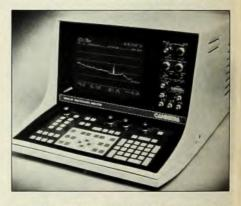
sors. Overall system control is provided by the multitasking software system. The use of dual bus architecture allows the instruments to be expanded to 16k data channels plus 65 kilobytes of program memory. A selection of signal processing modules allows the analyzers to be configured to meet specific requirements. A 12-in. cathode ray tube is used for display.—Canberra Industries, Inc., 45 Gracey Ave., Meriden, CT 06450.
