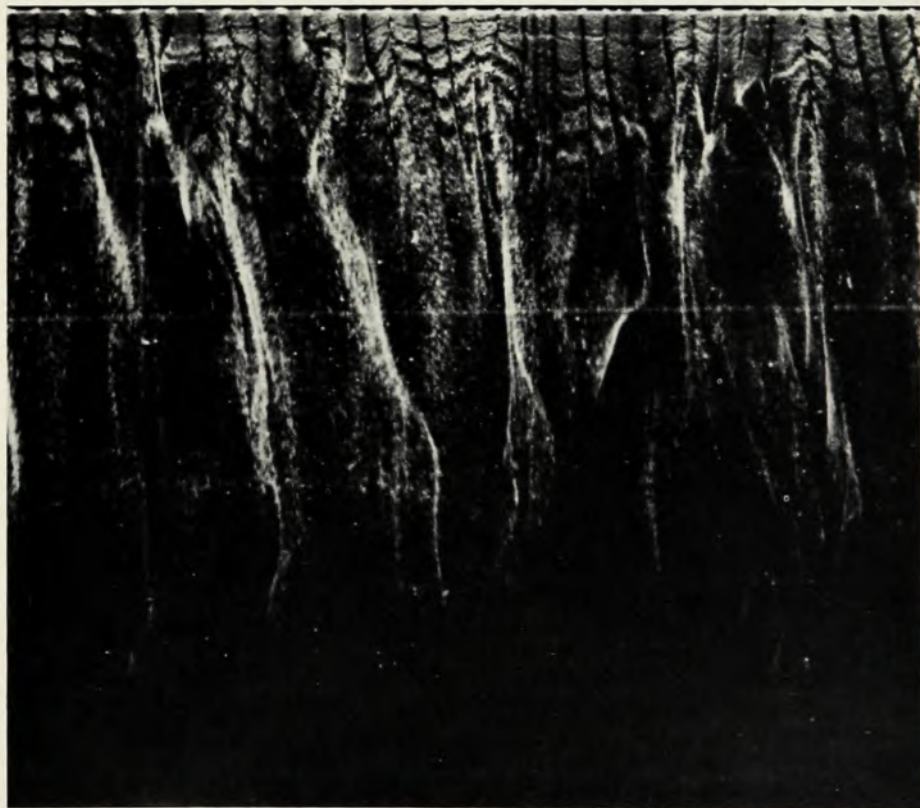
Turbulent boundary layer in water. Electrolysis (see wire at top of photo) produces tiny hydrogen bubbles, which act as tracers for turbulence phenomena. Note that the interrupted ribbons of bubbles quickly lose their orderly pattern as the fluid streaks "burst." Photo seen here is from the work of Steven Kline and his colleagues at Stanford University.
