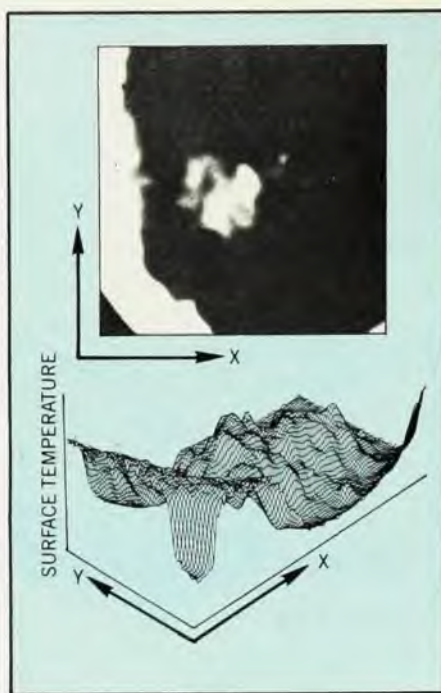
Infrared image of eroded refractory lining of a steel pipe and the corresponding isometric temperature profiles. The image covers an area of 2500 mm 2 and the temperature range is approximately 30–100°C. (Courtesy W. A. Ellingson.)
