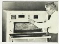
inates the need-to split thick samples and to extrapolate results. Measurements are completed in from 30 min to 1 h; the instrument can operate unattended. Accuracy is stated to be  $\pm 2\%$  and repeatability  $\pm 1\%$ . The instrument incorporates an integrating heat flow transducer. All measurements are made a 75°F mean temperature. Readings provided by the instrument are used to calculate R-value of the insulation.—Dynatech Corporation, 99 Erie St., Cambridge, MA 02139.
