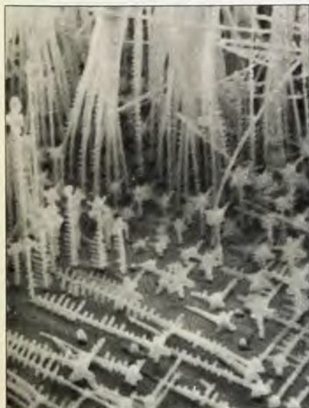
A cobalt alloy with a secondary phase of filamentary silica (emissive mode). Photo reproduced from R. Barlow and P. J. Grundy, J. Mater. Sci. , 1970, 5, 1005, with kind permission of Chapman and Hall, Ltd.
