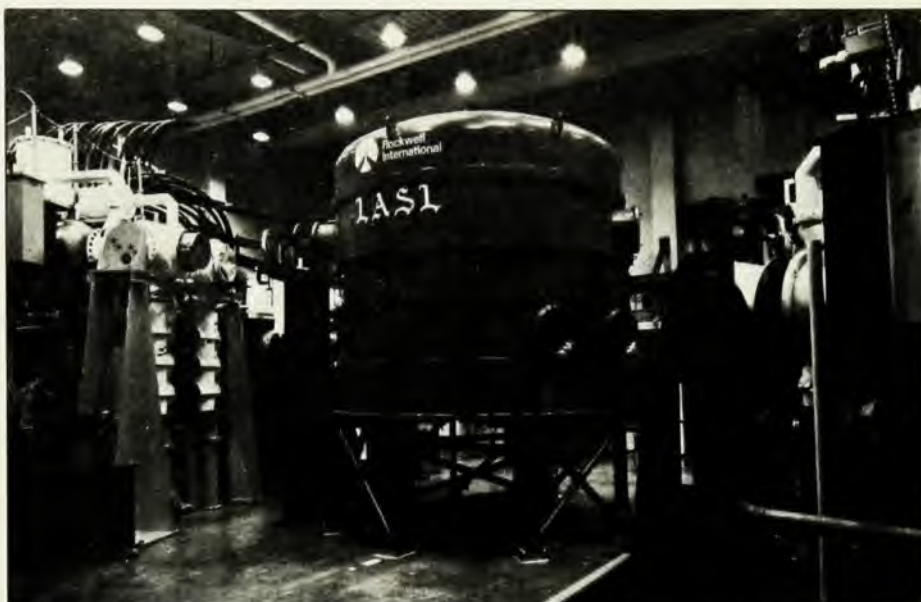
The 10-kilojoule Eight Beam System shown here during assembly at Los Alamos consists of four two-beam modules in an array around the centrally located target chamber. This system uses the highest-power carbon-dioxide laser ever built. Its high energy capability will permit experiments in a region of pellet gain far beyond current levels. Figure 4
