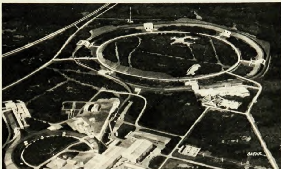
Isabelle. The 400 GeV \times 400 GeV proton-proton colliding-beam accelerator that DOE plans to construct at Brookhaven is at the upper right of this artist's drawing. Six experimental areas surround it. The linac and Alternating Gradient Synchrotron are at the lower left of photo.
