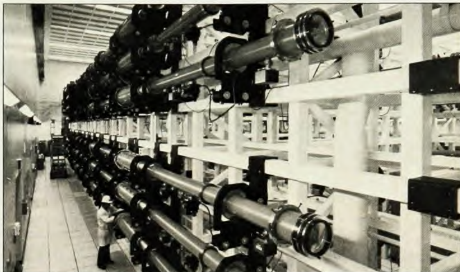
The Shiva laser-fusion facility at Lawrence Livermore Laboratory incorporates twenty neodymium-glass laser beams with total power likely to reach 30 terawatts. The cover of this issue shows the target chamber where all beams will be focussed. This photograph shows six beam lines.
