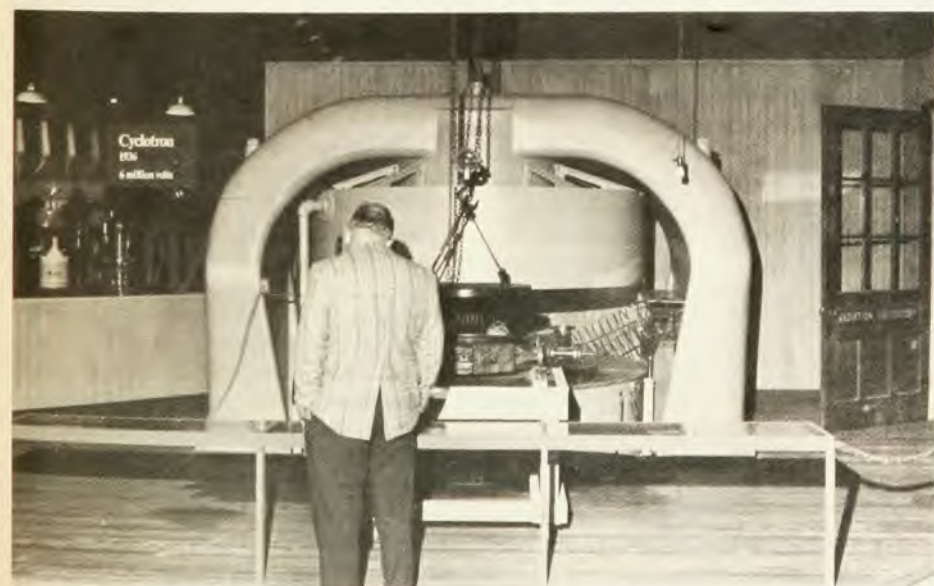
The 27-inch cyclotron. This historic accelerator, built by Ernest O. Lawrence and his associates in the 1930's, is featured in the recently opened Smithsonian "Atom Smashers: Fifty Years" exhibit. It is set up with the last vacuum chamber installed and a simulation of the 74-ton magnet yoke in a reconstruction of the Berkeley Radiation Laboratory. (Photo: Fermilab.)
