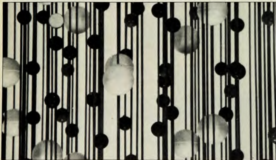
Model of part of the unit cell of Th_4H_{15} . The crystal structure, whose unit cell contains four formula units, was first proposed by W. H. Zachariasen in 1953 on the basis of x-ray diffraction measurements that yield only the symmetry and spacing of the thorium atoms. Recent neutron diffraction measurements by Mel Mueller and his coworkers confirmed this structure. Figure 6
