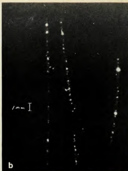
Ru 106 decay electrons in the chamber. At 150 psia of a Ne-He mixture, and no image intensification (a) several flares (bright areas) develop. Track length here is 4 cm. To reduce flaring, operation at lower total ionization per streamer was attempted (b). Here chamber pressure is 230 psia, and image intensification is 100. In both cases, pulses were 140 kV. Figure 6
