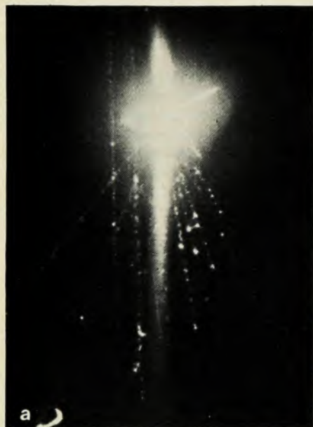
Negative pion interacting in chamber. Heavily ionizing nuclear fragments from this 200-GeV pion also cause flares (a). To cure this problem, microchannel image intensifiers were added to increase optical gain. Improved photo (b) was taken with 18-mm diameter microchannel intensifier, with gain of 10 000. Pressure was 370 psia. Figure 7
